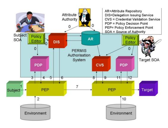
Figure 2. Components of the PERMIS Authorization System
